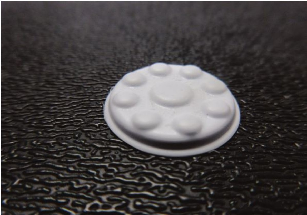
TOP VIEW OF FLANGE AFTER FINAL SANDING.
