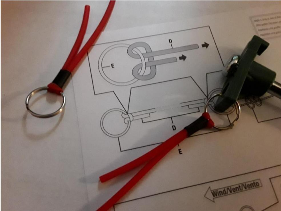
I found by tying the knot using some soapy water, the knot stays tight, however I added some short pieces of heat shrink pulled up to the knot. The extra Security seemed worth it.
