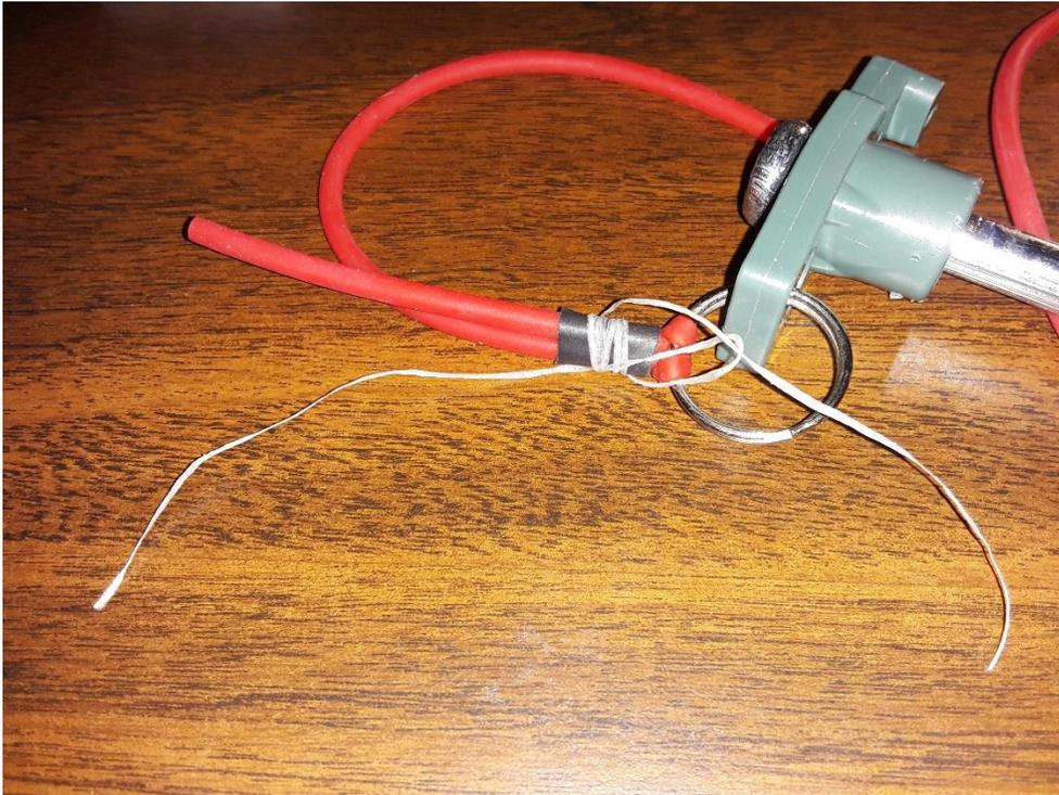
Using the Waxed Dental Floss I tied a 5 wind Cinch Knot over the Heat Shrink protecting the Silicone from cuts by the Floss.
