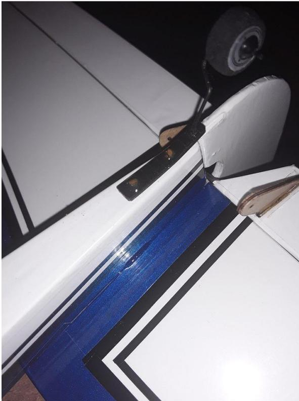
I used a little epoxy to glue the toothpicks on this assembly. I stuff a little epoxy in the holes first, then push the toothpick in through the tie wrap bracket. Trim and add a dab of epoxy to the top of each pin.
