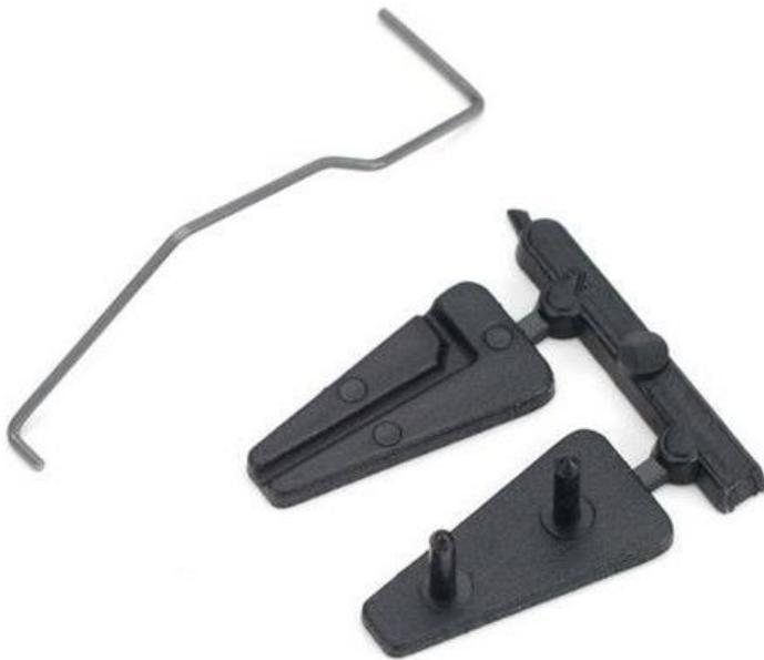
Alternately there is a mini/micro Du-Bro DUB854 tail wheel bracket available through WN. Using only the part with the pins you will need to drill a hole at the narrow end for the gear leg and fabricate the wire to connect to Rudder for steering.
