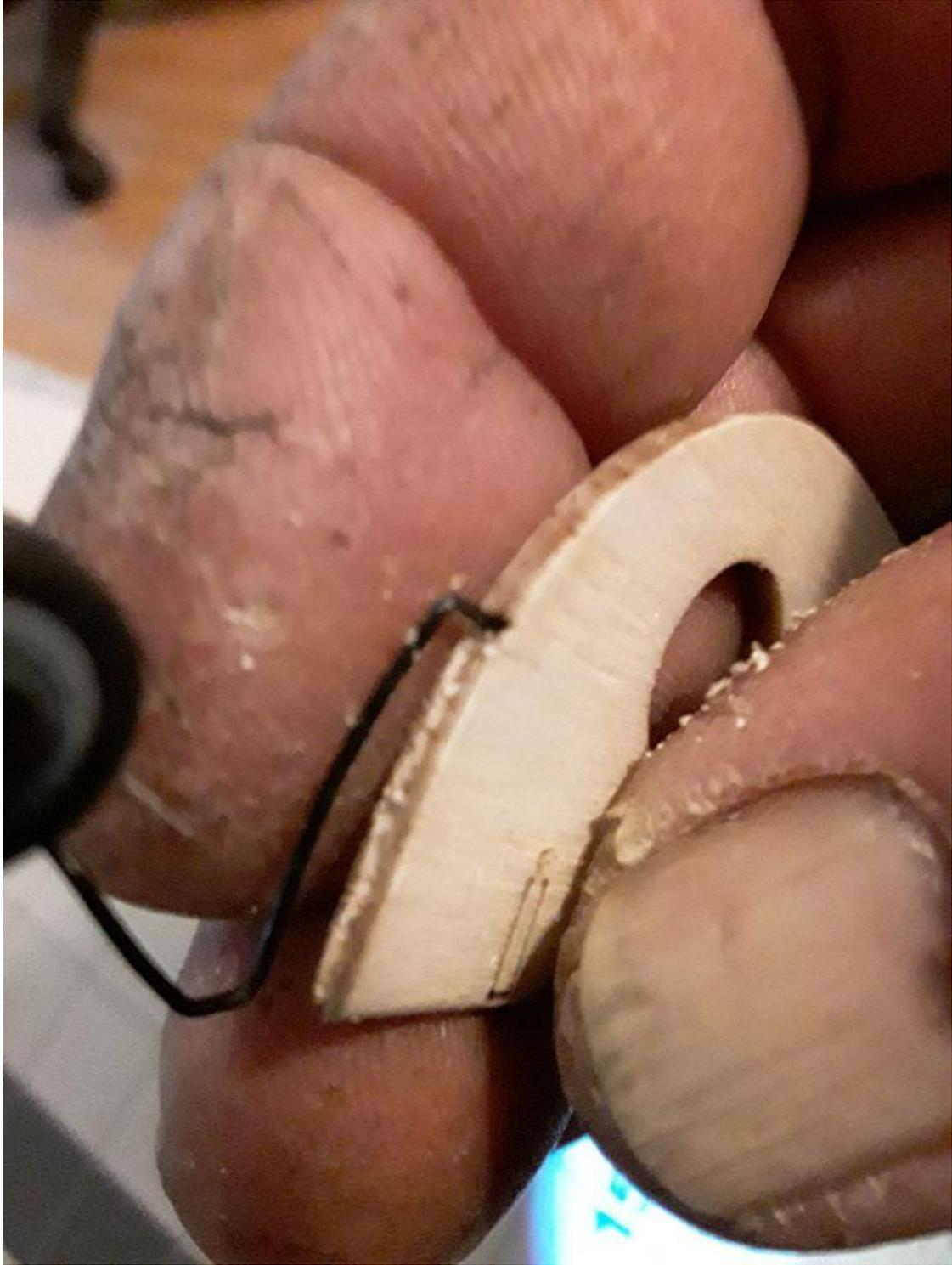
As shown in the picture, a small groove is made in the rudder and a hole is drilled. A small amount of epoxy pushed into the hole and bedding the wire in the groove hold it in place.
