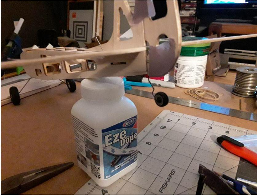
Shown mocked up on the WN Jr Falcon, the small bracket made from zip tie. This setup works quite well and acts as a lower hinge for the Rudder, and as a bonus weigh about nothing.
