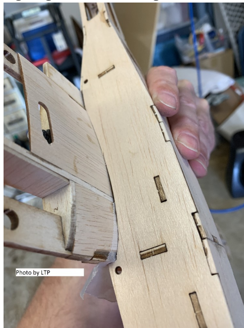
Figure 9 & 10 - Aligning Wing – Gluing Leading Edge Mount to wing
