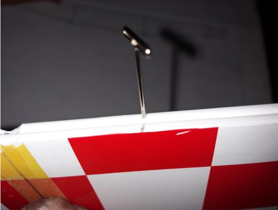
Aligning the holes centered on the Surface edge is key to a nice hinge line. Some people can “eyeball” the location very well.
