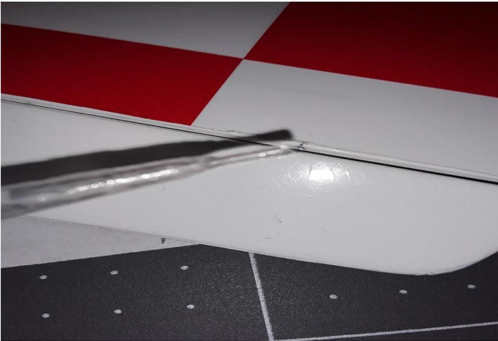
Flex the surface to ensure easy movement and do a pull test to ensure you have good adhesion. Congratulations! You have installed fishing line hinges!
