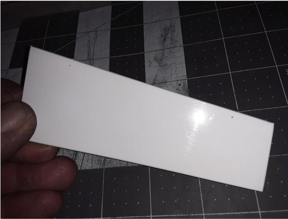
I've found that putting a second cross hole approximately  $3/16$ " from the edge and intersecting with the Hinge hole makes it a lot easier to apply the adhesive and keeps the CA out of the hinge line. You can see the holes in the picture above.
