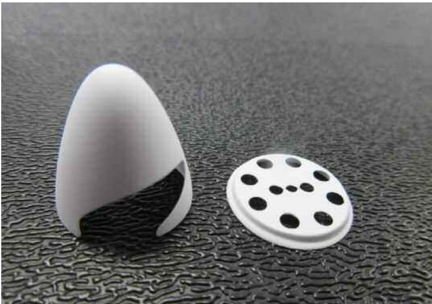
FINISHED 1104 SPINNER AND BACK PLATE.
