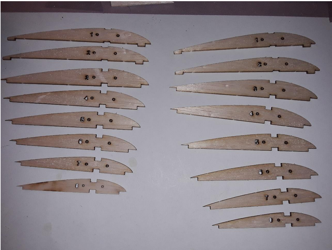
This picture shows the Ribs are numbered and laid out in order.
