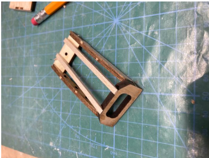
Lower air vent assembly. Glued to wing for bolt assembly
